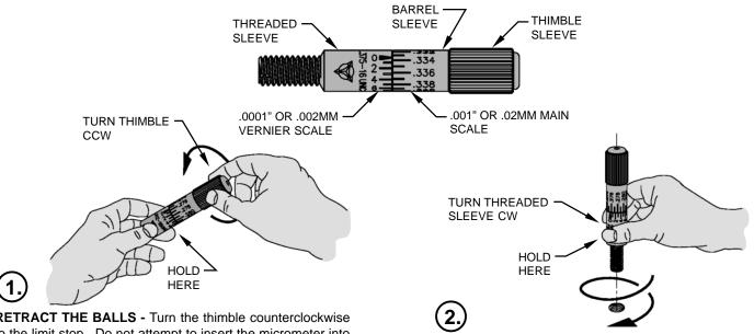
RETRACT THE BALLS - Turn the thimble counterclockwise to the limit stop. Do not attempt to insert the micrometer into the part without first retracting the balls.
