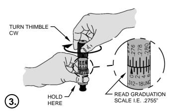
ENGAGE THE BALLS - Hold the threaded sleeve to prevent it from moving and then turn the thimble clockwise until it slips.
