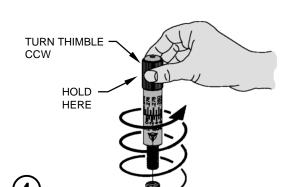
INSERT INTO THE HOLE - Hold the micrometer on the
