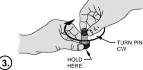
ENGAGE THE BALLS - Hold the threaded sleeve to prevent it from moving and then turn the pin clockwise until snug.
