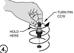
**REMOVE -** Turn the pin counterclockwise until the gage is removed from the hole.
